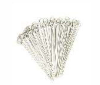
TMC 047 NICHROME LOOP Size: Dia 1.3 double wound , calibrated to 1.0 µl
