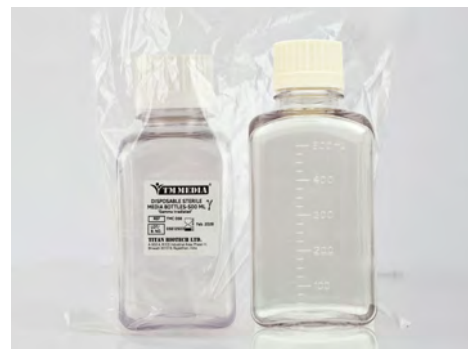
TMC 056 DISPOSABLE STERILE MEDIA BOTTLES 500 ML Alternative to Glass Media Bottles, Square (PETG), graduated bottles, sterilized by \gamma -Irradiation
