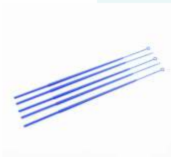
TMC 006 STERILE DISPOSABLE LOOP (ABS) Size: Inner Diameter 0.7 mm, Outer Diameter 2.1 mm, Loop calibrated to 1 µl Pack of 50 Loops Pack Size: 5*10 Nos
